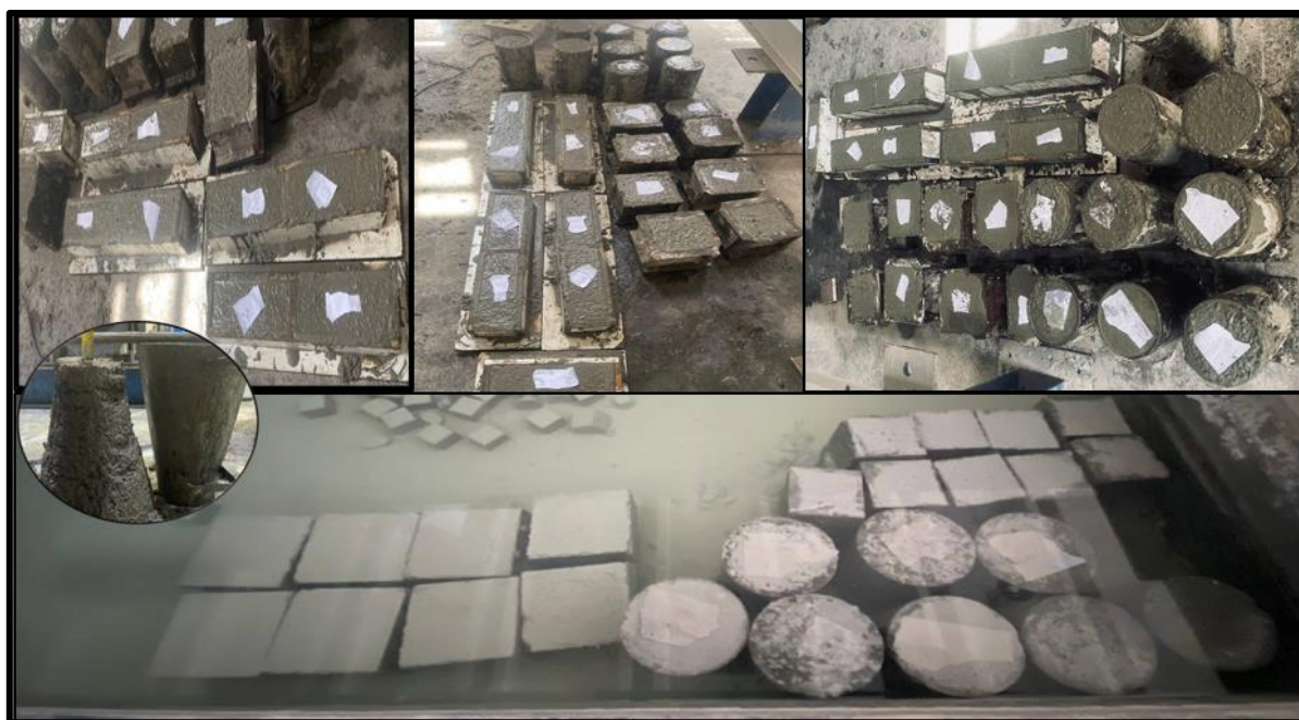
Figure (4): Plain concrete mix production and sample preparation
