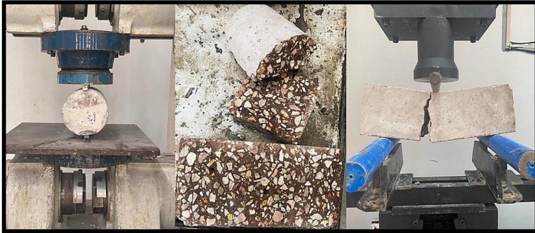
Figure (9): Tensile and flexural strength of zeo-concrete tests
