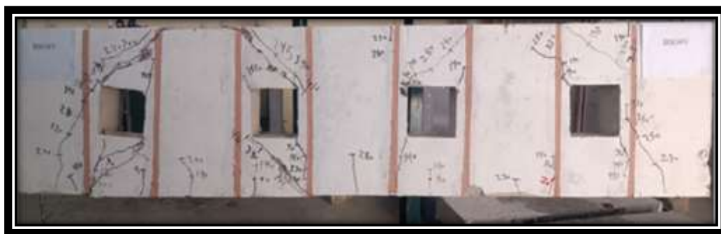
Figure (17): Crack patterns and failure mode for specimen (BSO4V)
