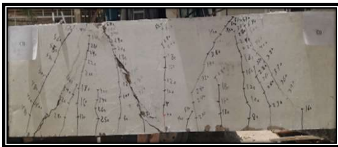
Figure (9): Cracks Patterns and failure mode for Control Specimen (CB Specimen)
