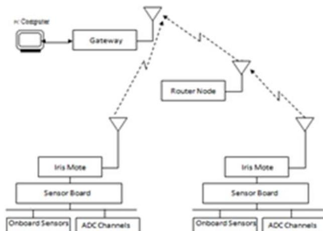
Fig. (2): Distributed controllers communication
