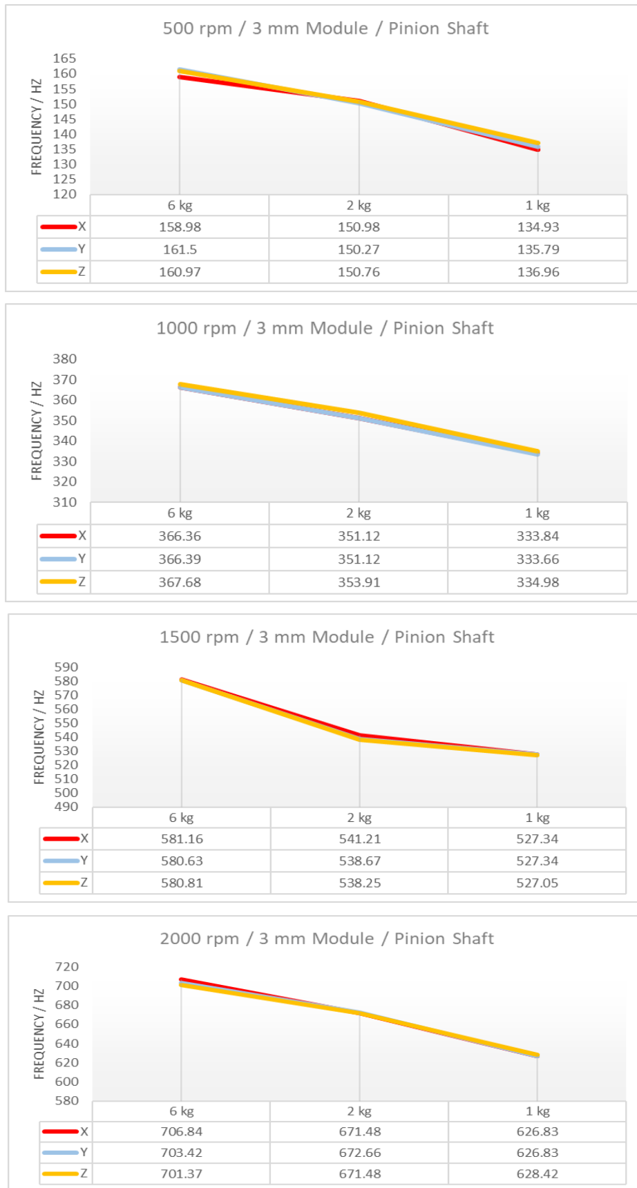
Figure 5. Relation between Loads and the Frequency for Pinion Shaft
